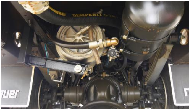
Underfloor installation: more compartment space for additional equipment or a portable pump
